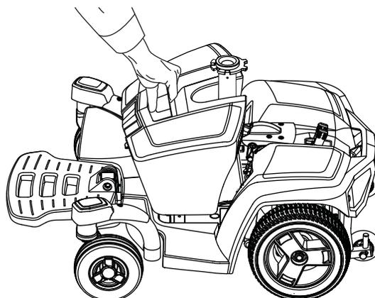
6. APPUYEZ SUR LE DOS DE LA BOÎTE DE LA BATTERIE VERS LE BAS JUSQU'À CE QU'IL SOIT FERMEMENT EN PLACE.
